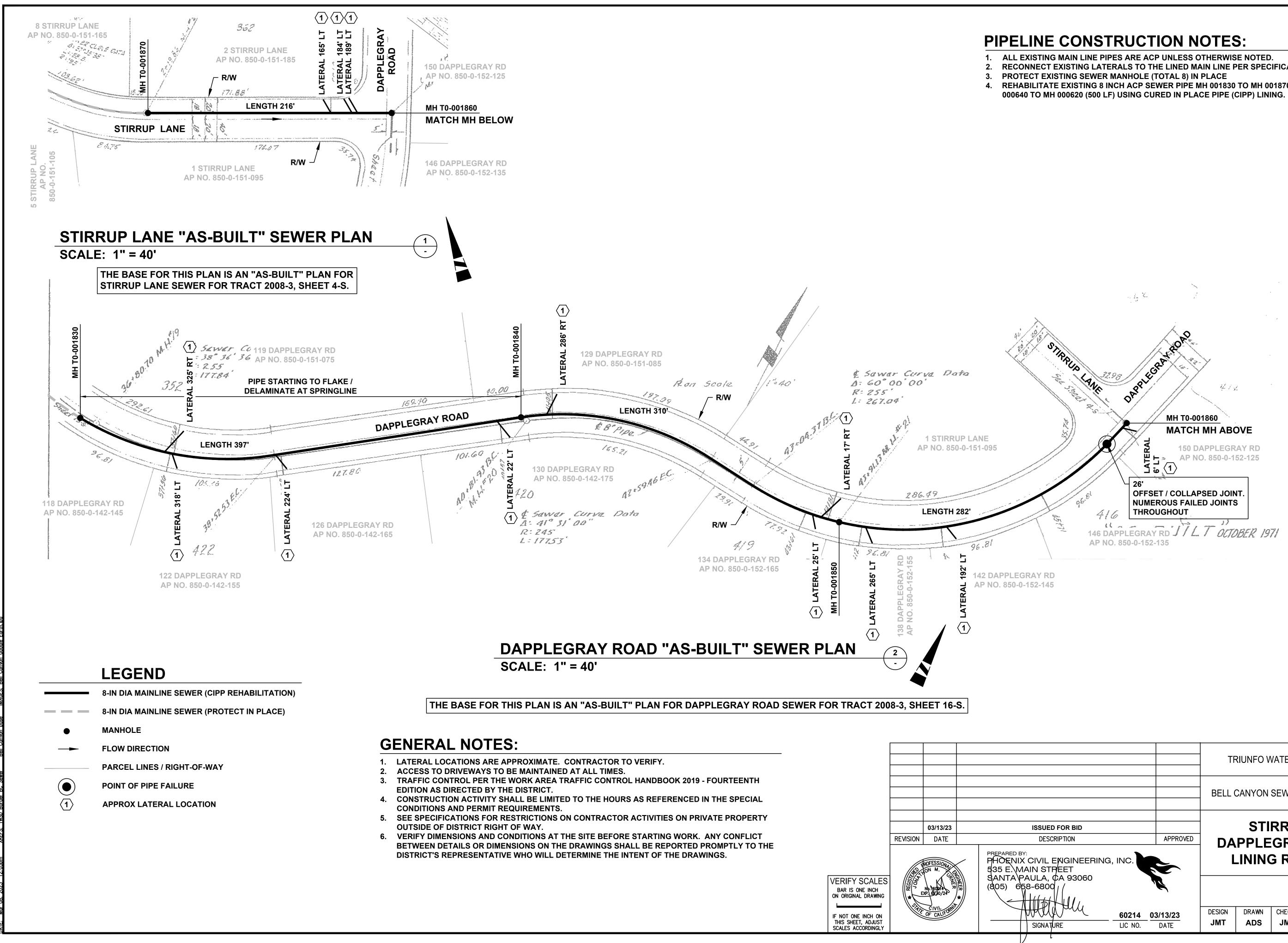
2. RECONNECT EXISTING LATERALS TO THE LINED MAIN LINE PER SPECIFICATIONS (TOTAL 22) 4. REHABILITATE EXISTING 8 INCH ACP SEWER PIPE MH 001830 TO MH 001870 (1205 LF) AND MH
